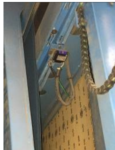
Adjustable photocell belt control system
