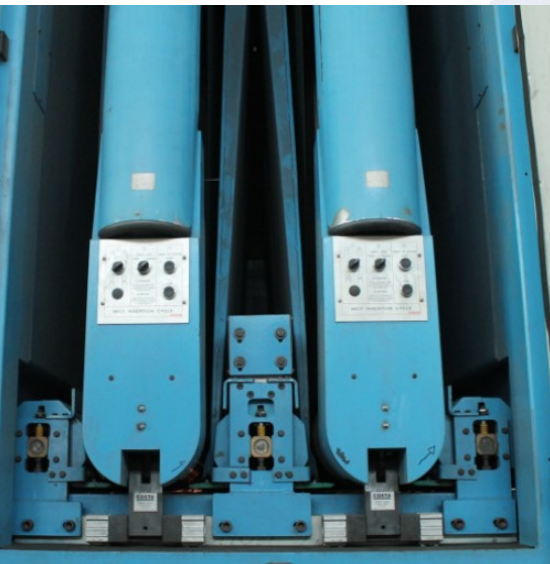
Quick automatic locking system for the two heads
