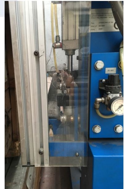
HOT WIRE SYSTEM to cut the PVC between the sheets
