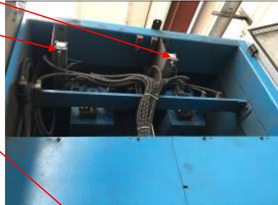
Cleaning system for abrasive belts
